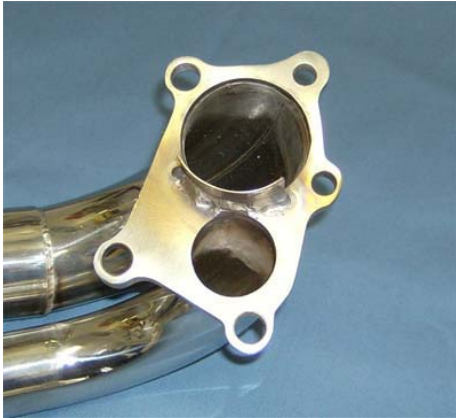
Divorced Downpipe Inlet
